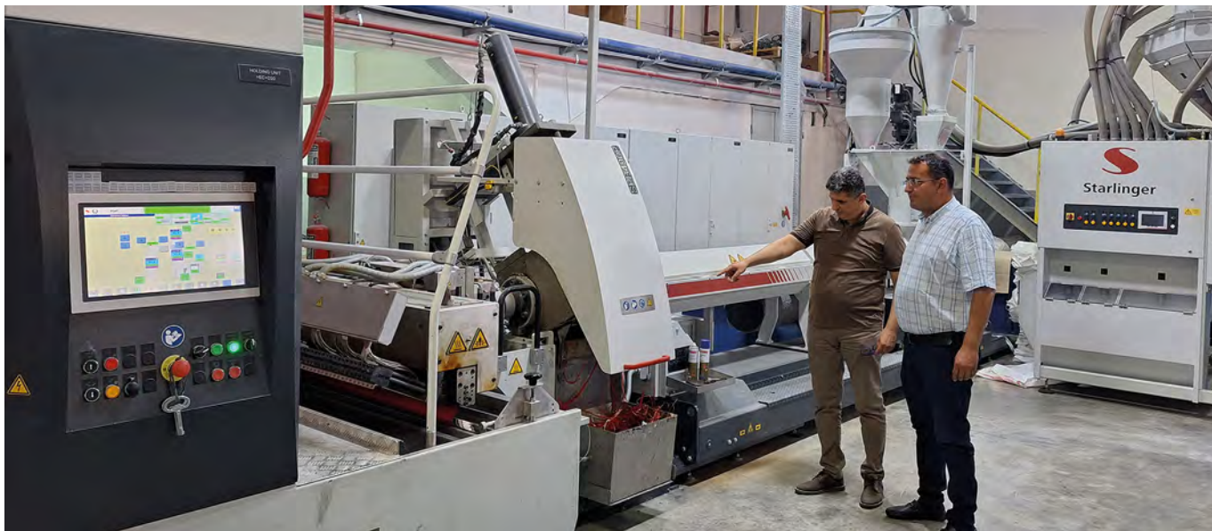
Using a Starlinger PP tape production line, Prof Sentetik produces PP tapes for FIBC fabric with recycled polypropylene (rPP)
