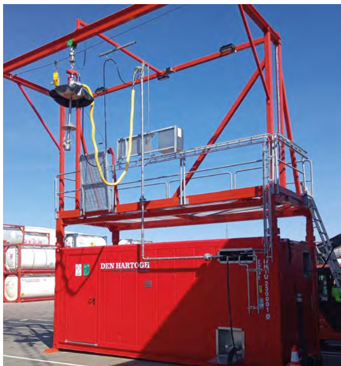
By using a heated batch with a chemical cleaning agent, the latex is dissolved in the tank, eliminating the need for manual work
