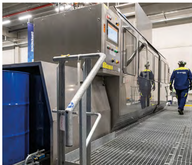
Van Moer's fully automatic lines are designed for filling a wide range of both toxic and non-toxic liquids
