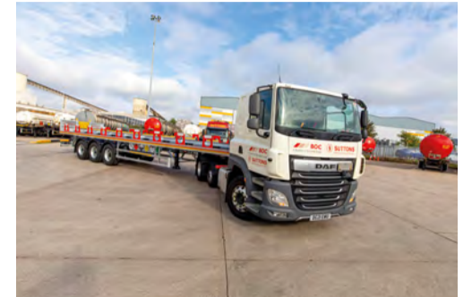
The new pintle trailers feature better positioning of the ADR marker boards
