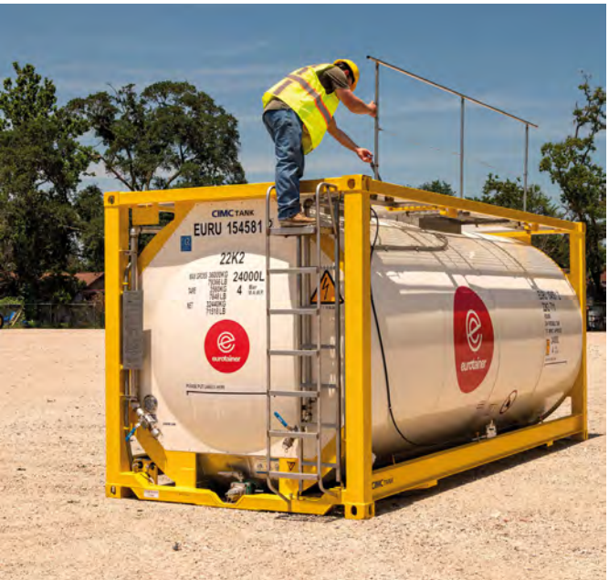
A collapsible handrail on top of the container provides fall protection for workers
