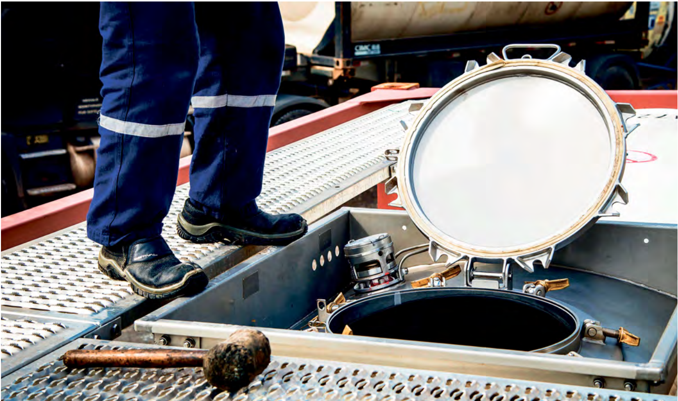
Access should only be allowed under a safe system or permit to work procedure and the supervision of a responsible person
