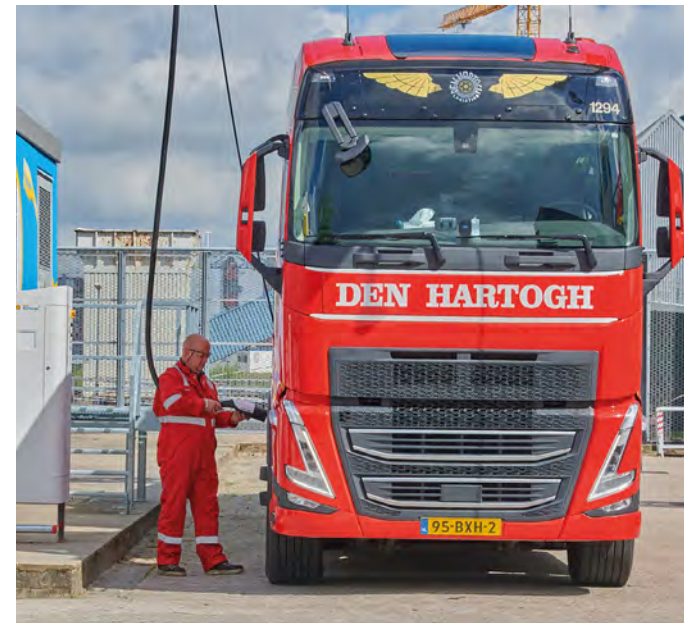
The megawatt charger means a truck with a 1 MWh battery can be fully charged in one to two hours
