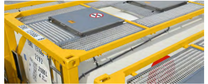
B Style walkways deliver a higher safety that increases the level of fall protection
