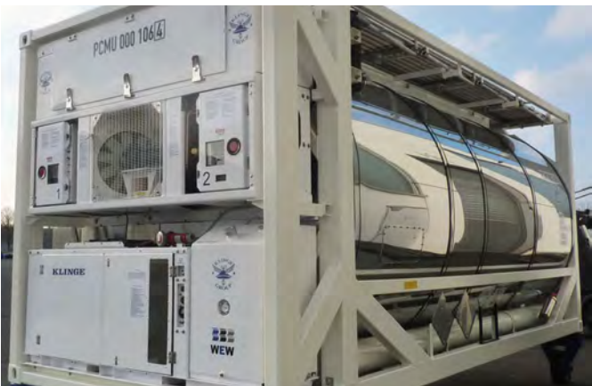
Klinge's dual refrigeration unit and genset
