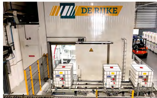
The Type 71 can fill a 1,000-litre IBC every two minutes
