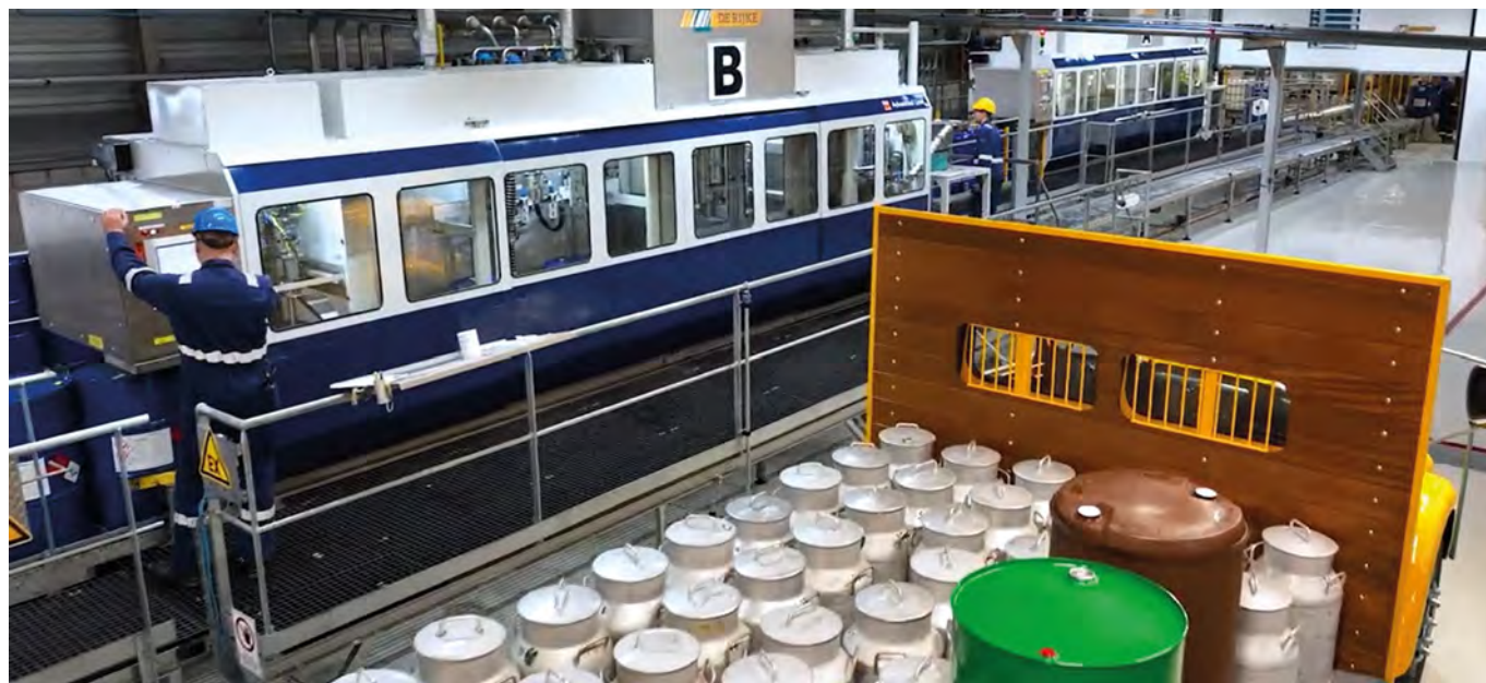
The latest Feige filling machines at De Rijke operate on a 'closed cabinet' basis
