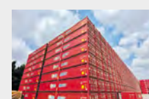
40ft half height container for steel bar &amp; coil and other dry cargoes (Total height of 3x40HH = Total height of 2x40GP)
