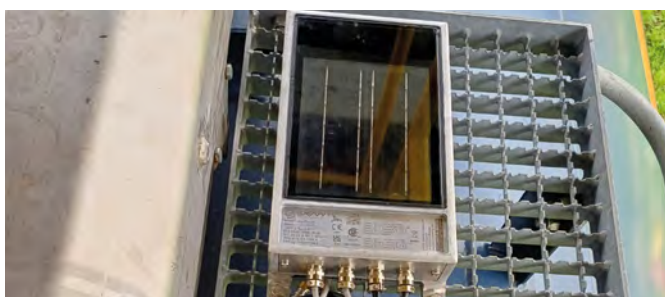
Working in tandem, the Savvy CargoTrac-Solar device and the TODO pressure cap sensor continuously monitor the securement of pressure caps
