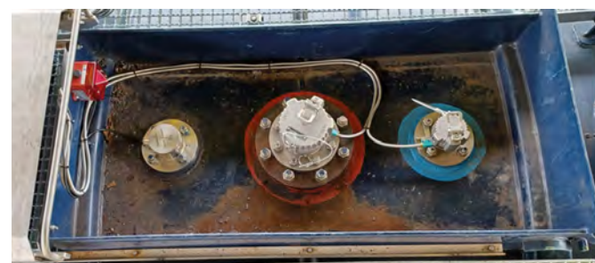
Working in tandem, the Savvy CargoTrac-Solar device and the TODO pressure cap sensor continuously monitor the securement of pressure caps
