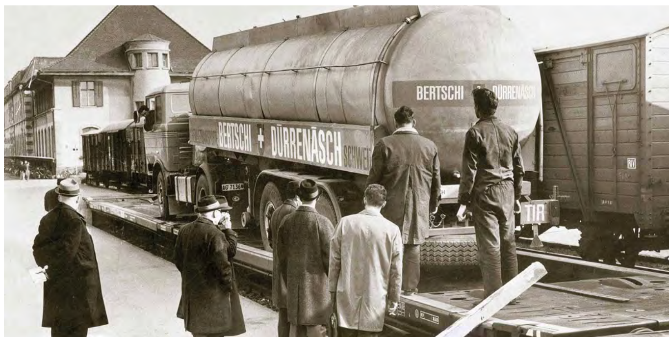
1967 - Hupac start-up with a chemical tank trailer on a newbuilt special rail-wagon for intermodal trailer transport
