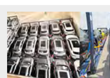
Foldable transport rack for passenger cars 12192*2438*270mm (foldable size) 15240*2438*2438mm (extendable size)
