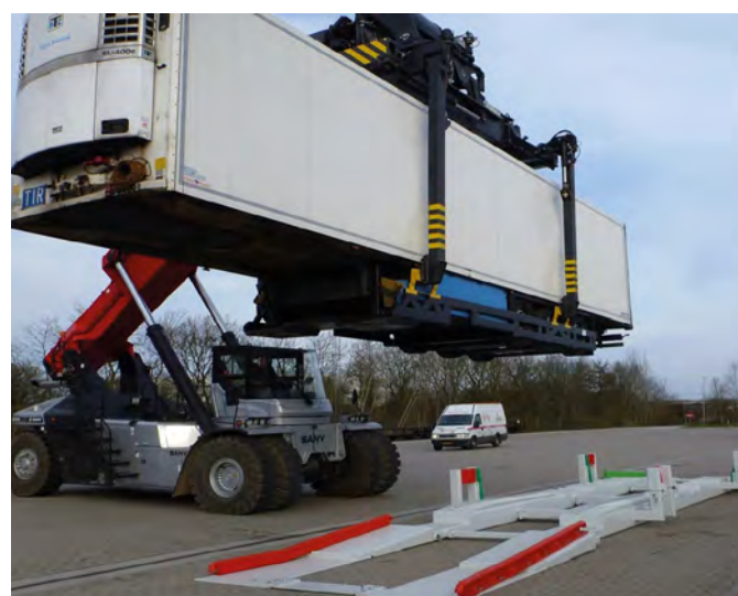
The NiKRASA system allows non-craneable trailers to be loaded onto the rails quickly and easily
