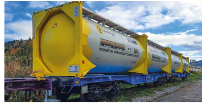
Four CemTainers can be carried on a 2x45 ft InnoWagon flatcar configuration
