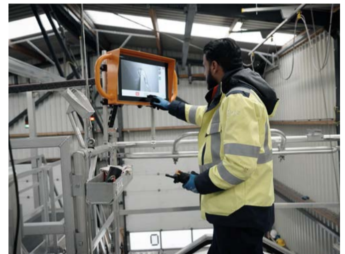
If contamination does occur, customers can retrieve the ScanTank file and rule out the tank trailer or container as the root cause
