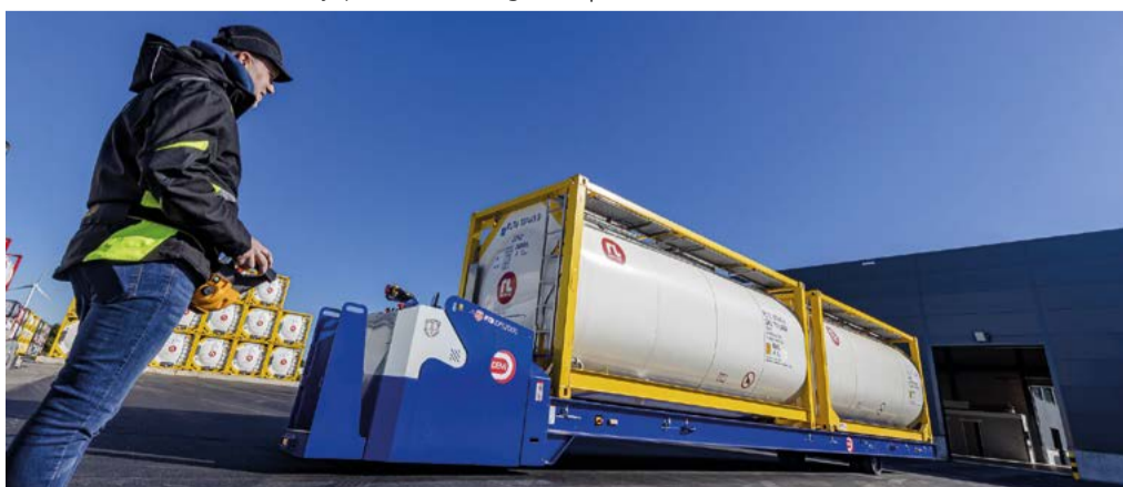
DEMI Netherlands took delivery of a rechargeable electric powered 'container mover' that can be operated by one person standing at the control centre and viewing a built-in forward camera or standing nearby with a separate portable controller
