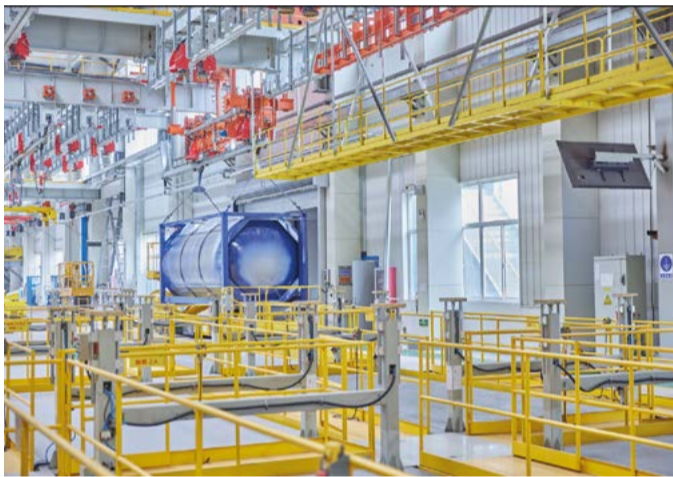
CIMC Safeway's powder coating line eliminates VOC emissions
