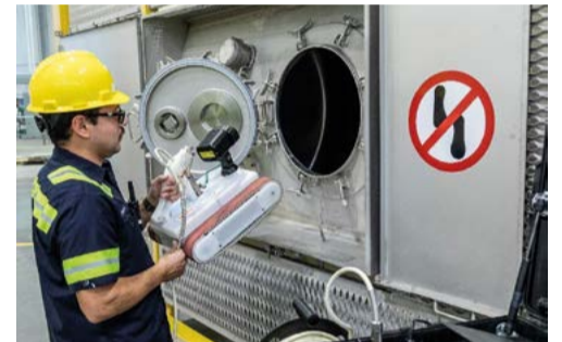
Robotics are used for internal inspections of tank containers
